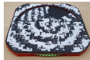
Figure 3: Example of a 3D printed controller with a detection pattern on it
